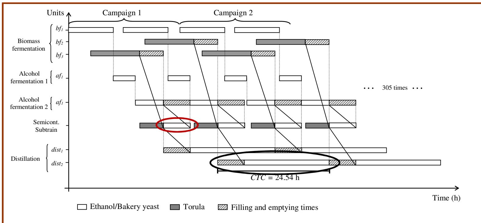
✓ Reduced idle time    ✓ Limiting cycle time – No idle time
